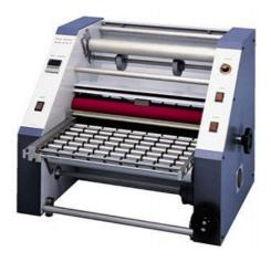
The RLM is a dry film laminator especially made for small companies, schools, research and development departments. All commercial laminates for PCB manufacture and mould-etching part technique can be processed. Due to adjustable pressure control and adjustable laminating speed, solder mask application is also possible without problems.
